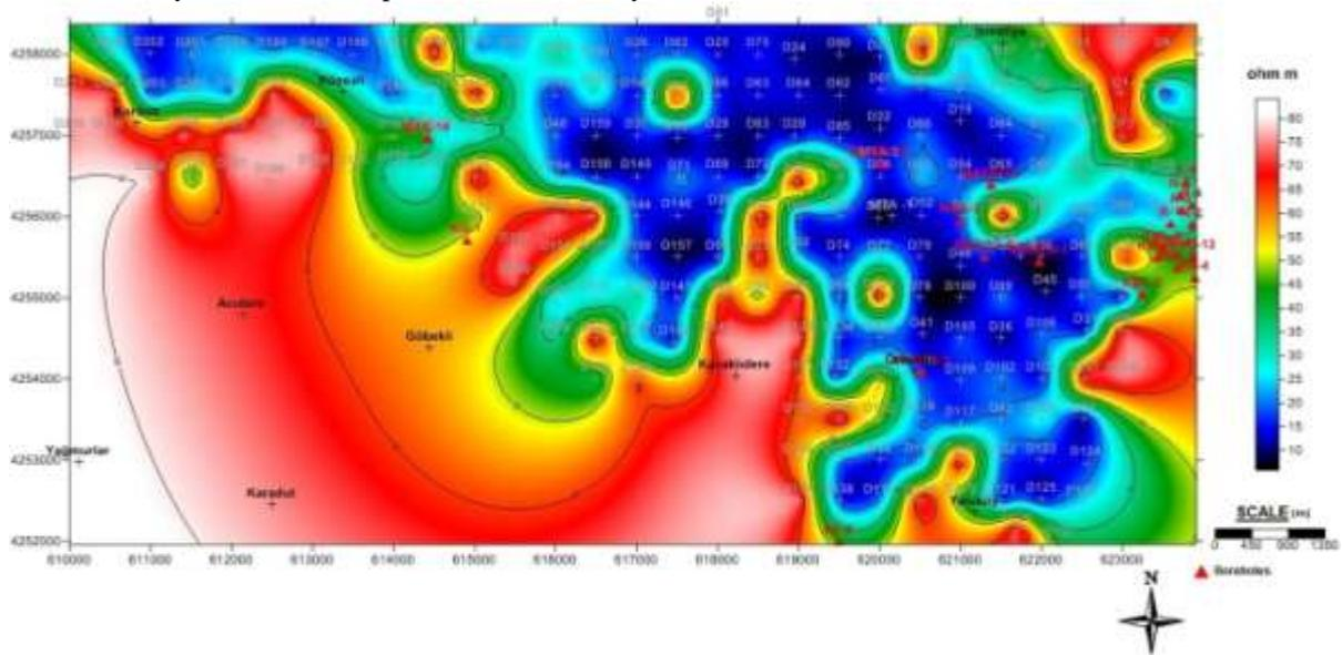
**Figure 13.** Resistivity depth map of AB/2 = 1600 meter
