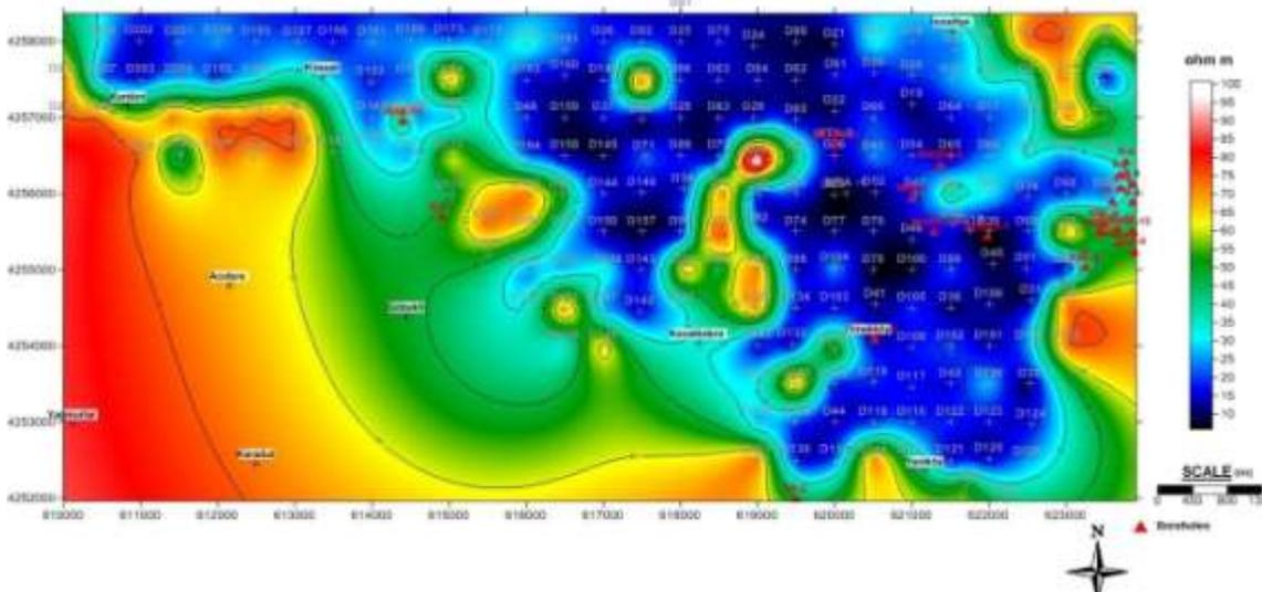
Figure 12. Resistivity depth map of AB/2 = 1500 meter
