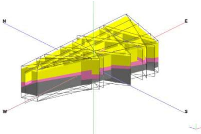
**Figure 43:** Fence diagram of resistivity and stratigraphy of the Kavaklıdere geothermal field
