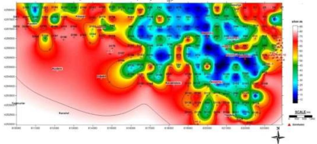
Figure 19. Resistivity depth map of  $AB/2 = 2100$  meter
