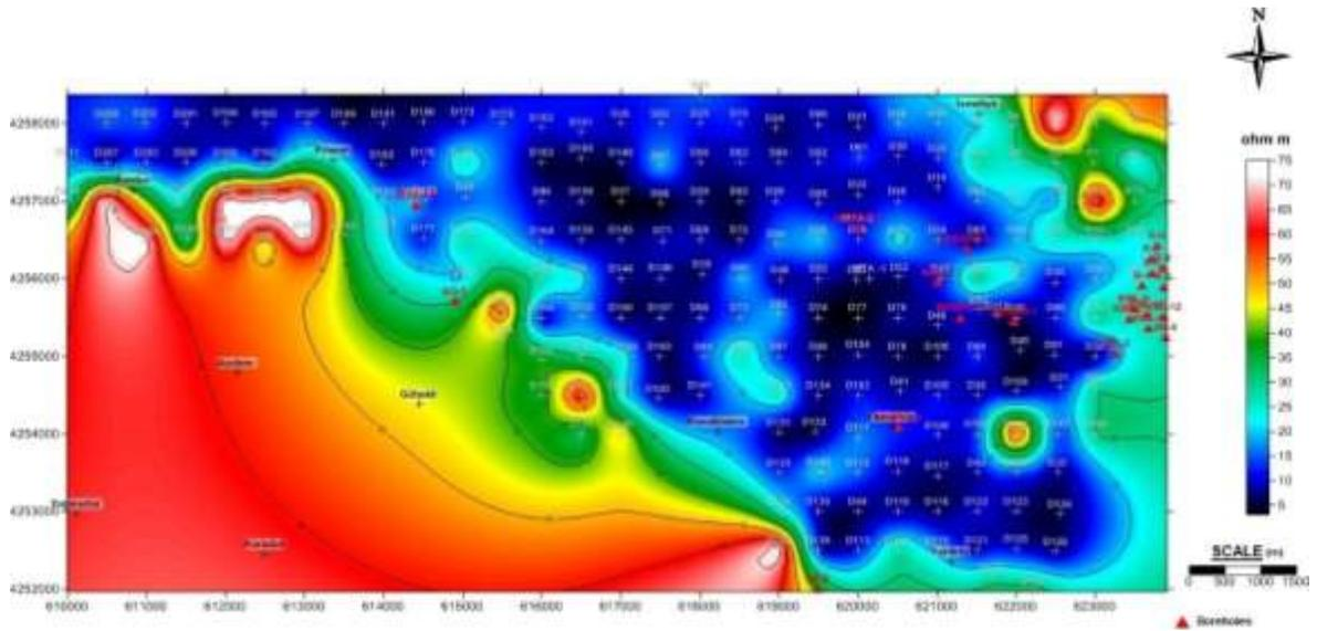
Figure 7. Resistivity depth map of AB/2 = 1100 meter
