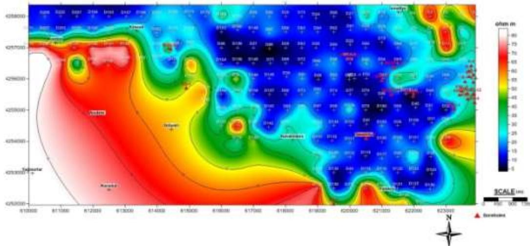
Figure 10. Resistivity depth map of AB/2 = 1300 meter
