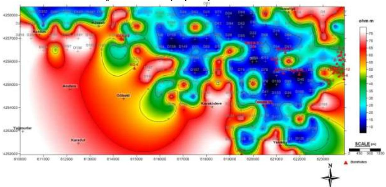
**Figure 14:** Resistivity depth map of AB/2 = 1700 meter
