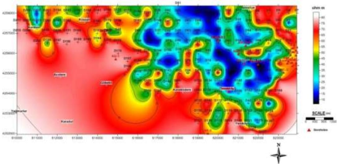
Figure 18. Resistivity depth map of  $AB/2 = 2000$  meter
