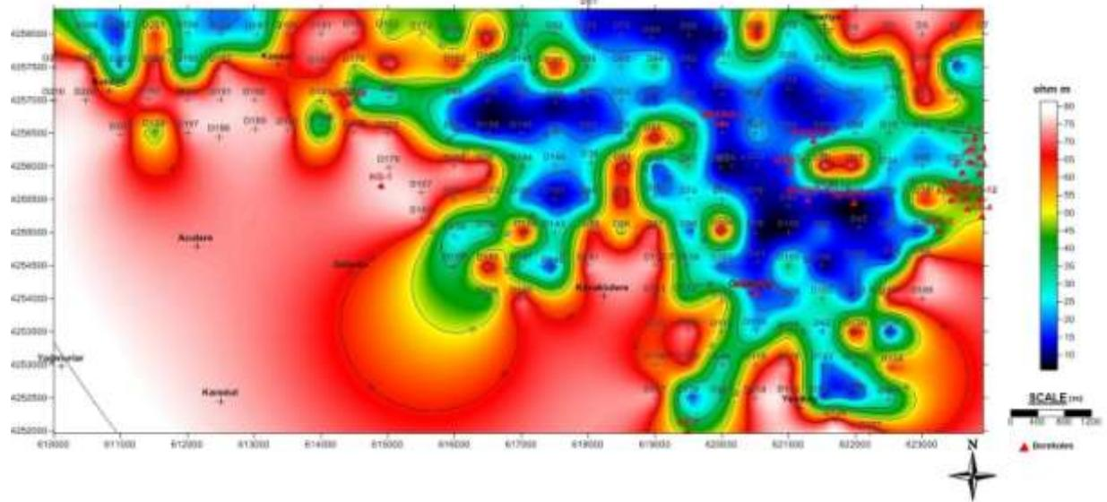
Figure 16. Resistivity depth map of AB/2 = 1800 meter
