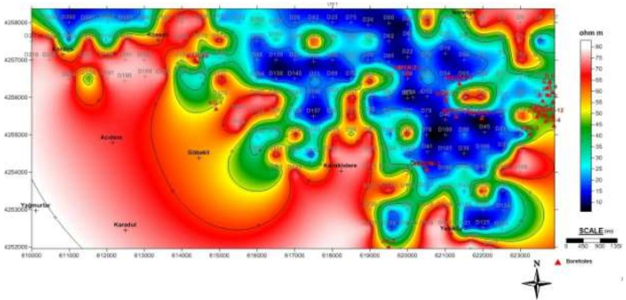
Figure 15. Resistivity depth map of AB/2 = 1750 meter
