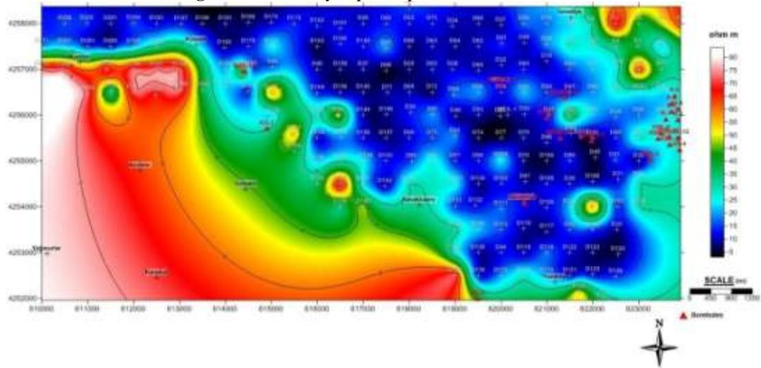
Figure 8. Resistivity depth map of AB/2 = 1200 meter
