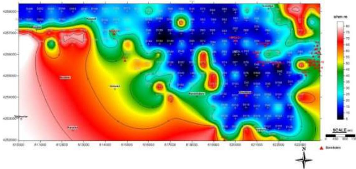
Figure 11. Resistivity depth map of AB/2 = 1400 meter
