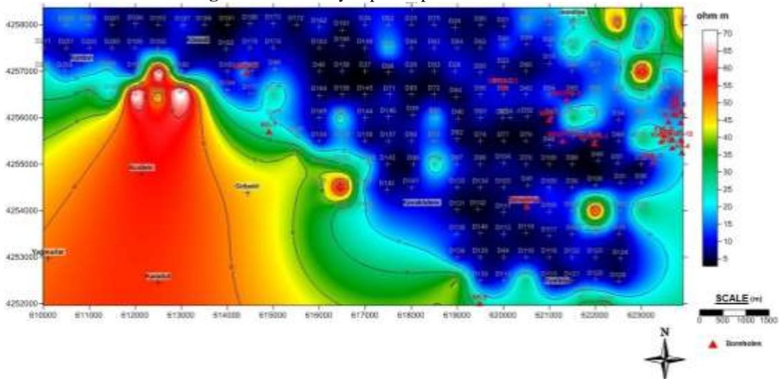
Figure 6. Resistivity depth map of  $AB/2 = 1000$  meter
