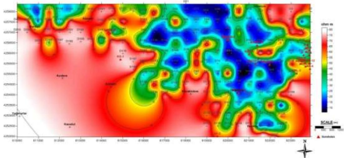
Figure 17. Resistivity depth map of AB/2 = 1900 meter
