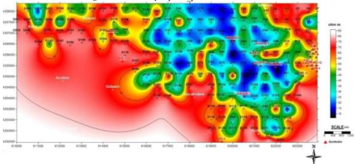
Figure 20. Resistivity depth map of  $AB/2 = 2200$  meter
