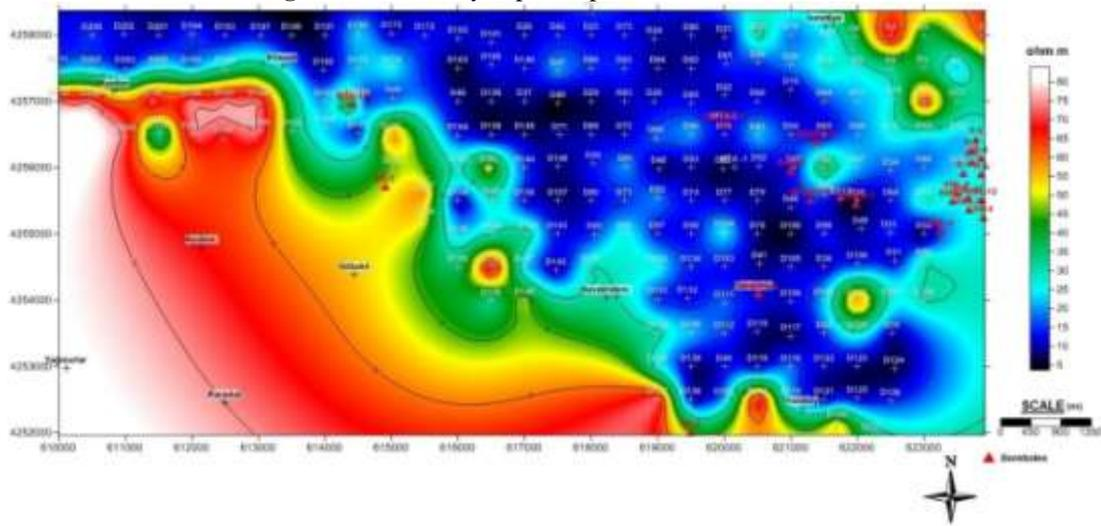
Figure 9. Resistivity depth map of AB/2 = 1250 meter
