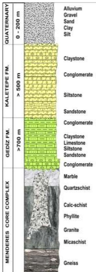
**Figure 3:** Simplified geological map and generalized stratigraphic vertical section of the Kavaklıdere geothermal field (Özdemir et al., 2016)
