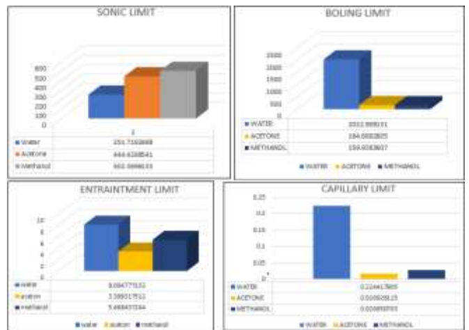
Figure 6: Comparison of different limits for different working fluids
