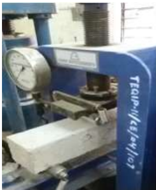
Figure 1: Test set up for flexural Test
