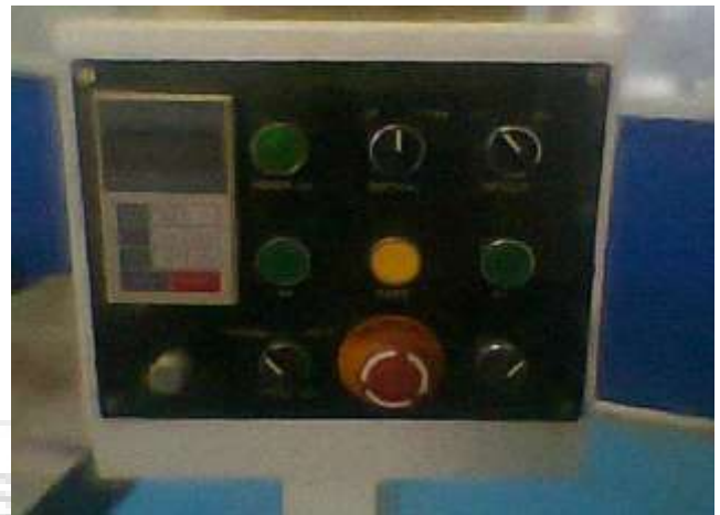
Figure 4: Control panel of friction stir welding equipment
