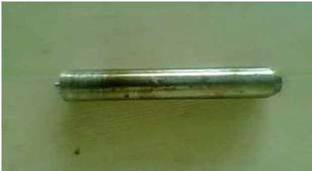
Figure 2: HSS Cylindrical profile tool
