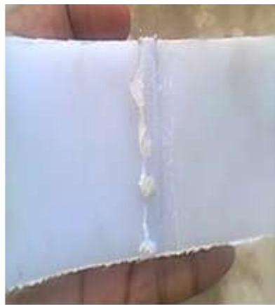
Rotational speed 750rpm Pin Diameter 4.2mm
