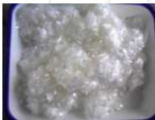
Fig. 2: Type of PVA fiber used in experiment (RMS702)
