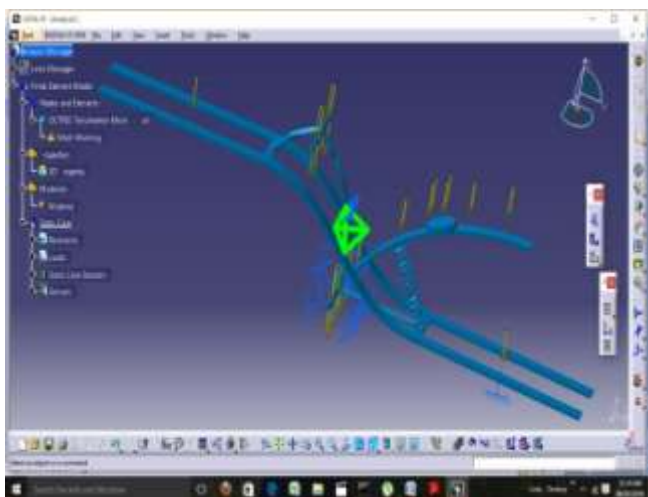
Figure E: Displacement pattern for aluminum chassis.
