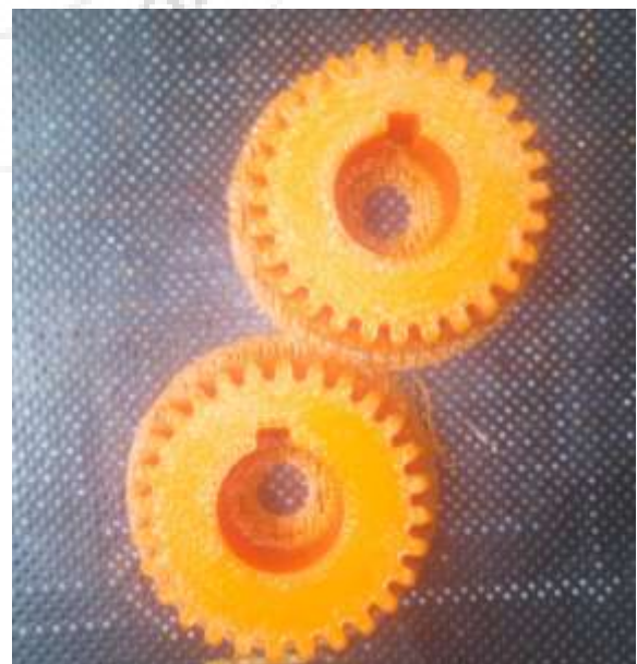
Figure 13: Gear Coupling Manufactured by FDM Process
