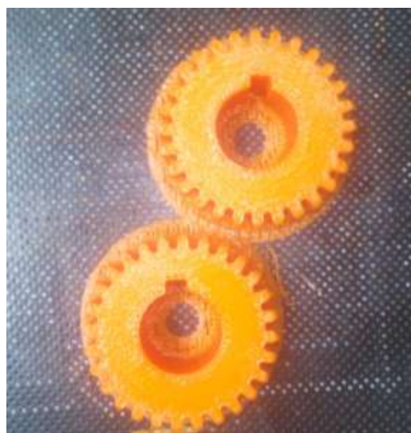
Figure 13: Gear Coupling Manufactured by FDM Process
