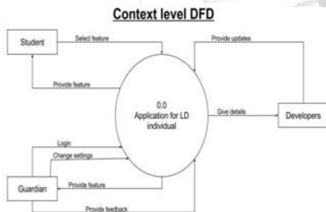
Figure 2: Context Level diagram of proposed system
