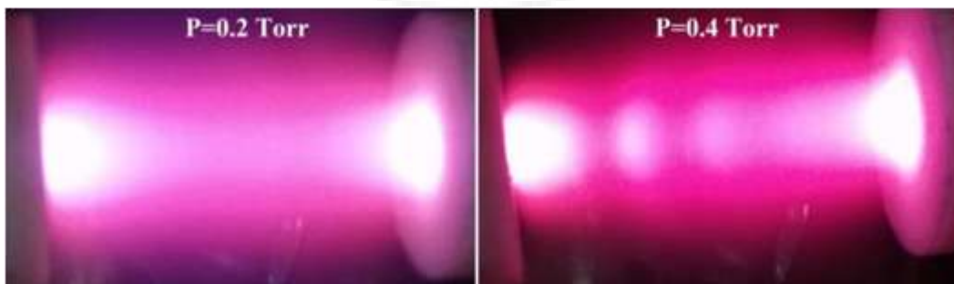
Figure 2: Effect of Ar gas pressure on the glow discharge structure of the hollow cathode system with 19 mm depth
