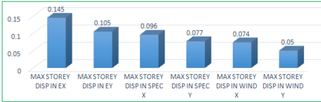
DISPLACEMENT OF RCC SHEAR WALL STRUCTURE WITHOUT P-DELTA EFFECT X -AXIS DISPLACEMENTS & Y-AXIS IN M Graph 1
