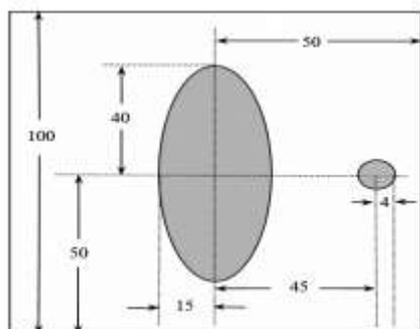
Figure 1: Schematic diagram of the template (unit: mm)
