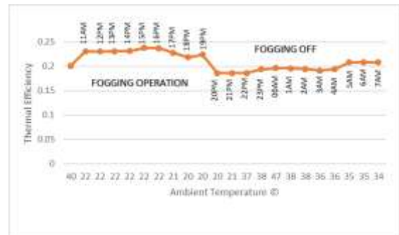
Figure 8: Thermal efficiency against ambient temperature during summer season
