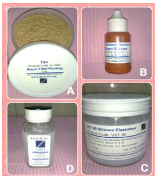
Figure 1: A: Rayon flocking (tan color), B: Burnt sienna (F1) pigment, C: VST 50 silicone base, D: VST 50 silicone catalyst
