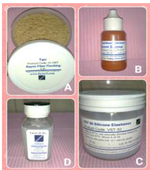
Figure 1: A: Rayon flocking (tan color), B: Burnt sienna (F1) pigment, C: VST 50 silicone base, D: VST 50 silicone catalyst
