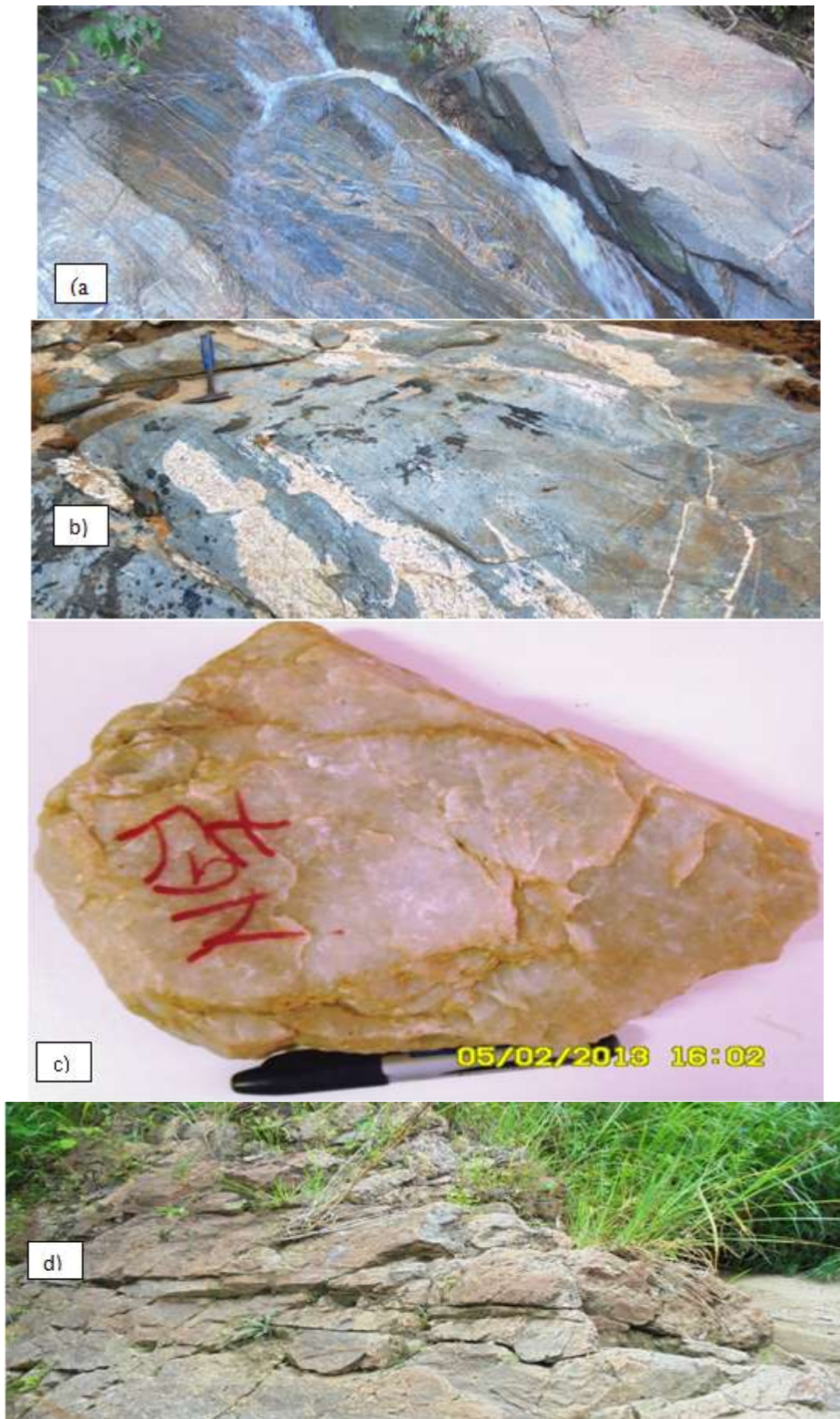
Figure 3: Pictures of potential rock source: a) Gneiss ;b) Amphibolite ; c)Quartzite; d) Granite
