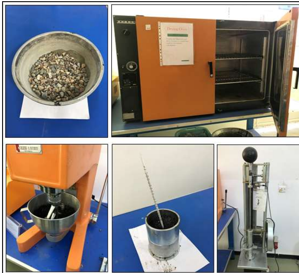
Figure 3: Procedure of Preparing Marshall Specimen
