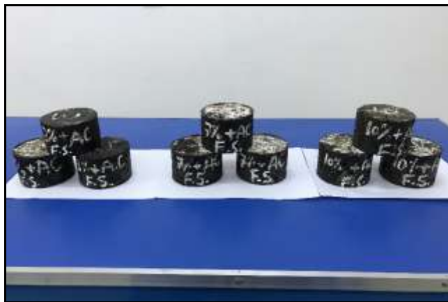
Figure 6: Modified Marshall Specimens with (F.S% + AC)
