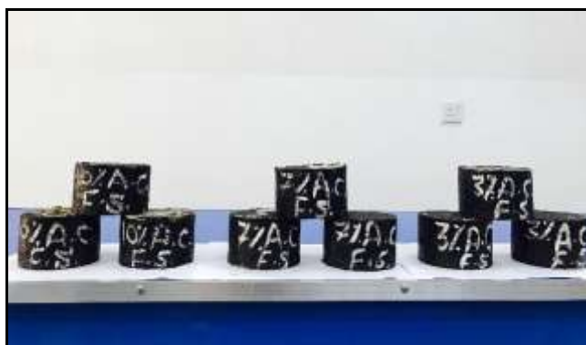
Figure 7: Modified Marshall specimens with (F.S% AC)
