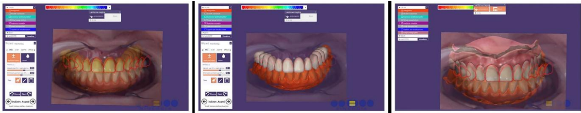
Figure 5: The dental technician used the outline of the virtual smile obtained to place a tooth from the library or to create customized teeth to convert the virtual 2D teeth arrangement into a 3D teeth arrangement
