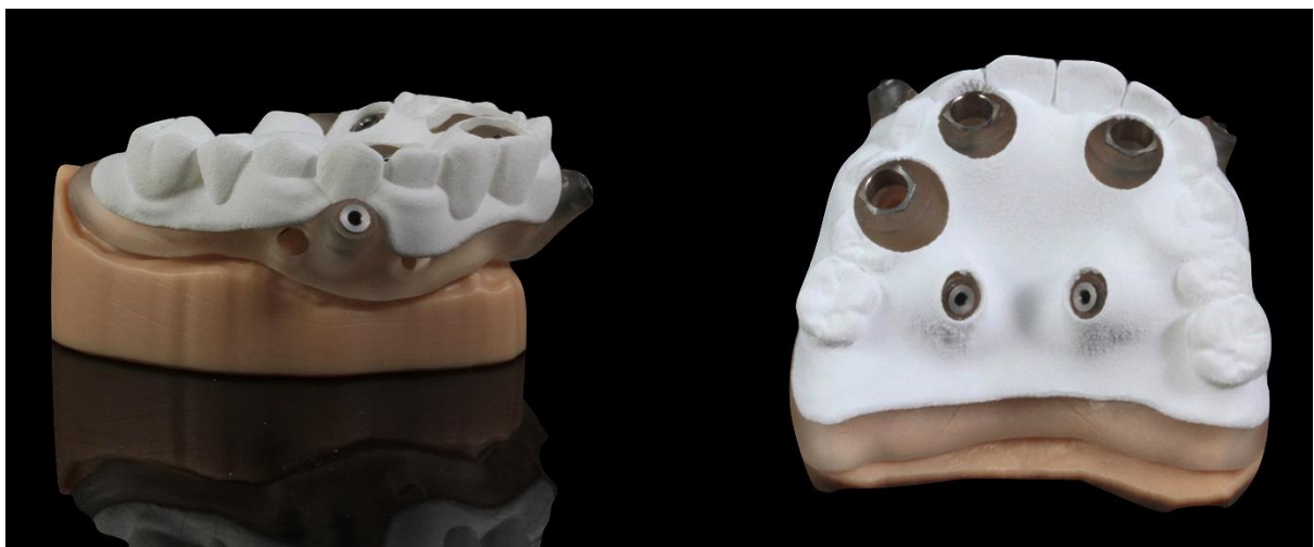
Figure 11: A stereolithographic surgical template was made with a rapid new prototyping technology.
