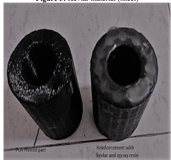
Figure 6: Part 3d printed with whole PLA (left) Part with reinforcements (right)
