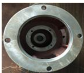
Figure 7: Corroded Base of the Casting
