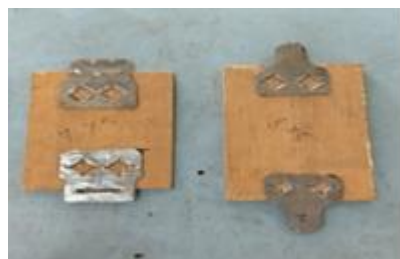
Figure 3: Clamps Fitted to the Plywood
