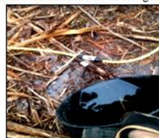
Pouring water onto stake/ground contact to ensure conductivity
