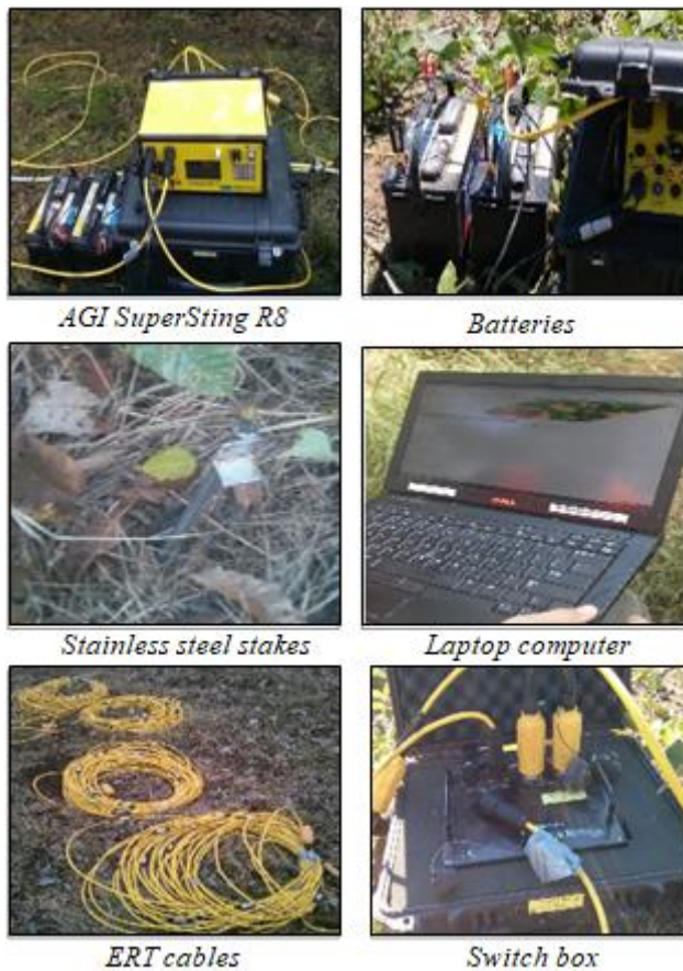
Figure 3: ERT data acquisition equipment.
