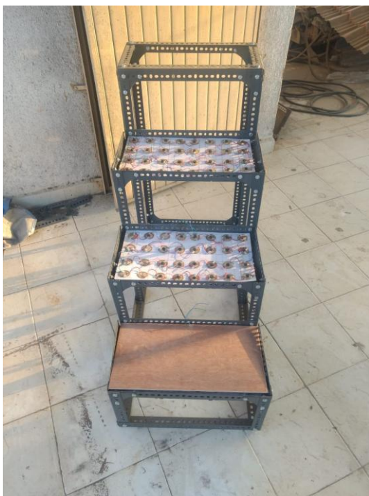
Figure 2: Arrangement of wooden plates over the sensors and movable springs
