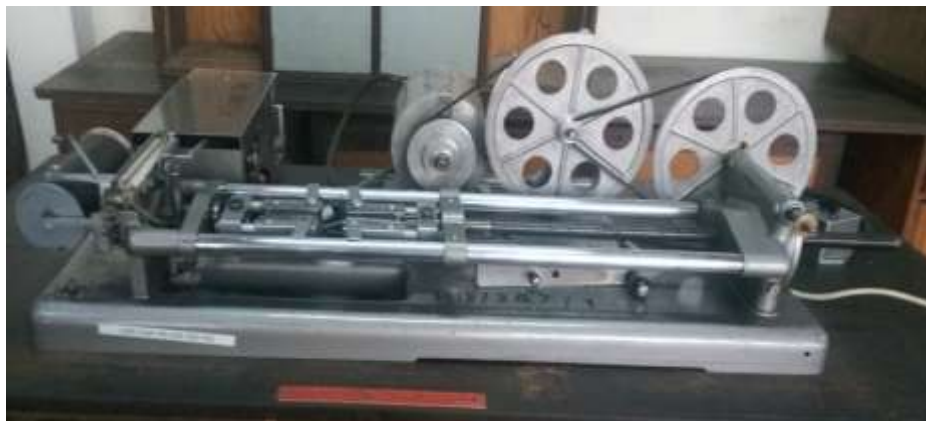
Figure 5: Tensile strength test machine for the determination of tensile force of fibre
