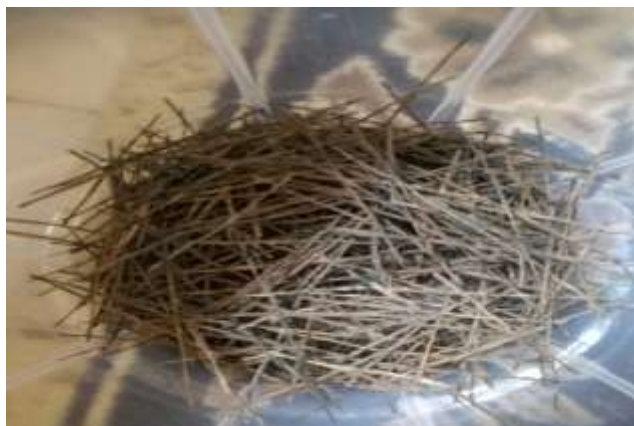
Figure 1: photography of untreated borassus aethiopum mart fibre
