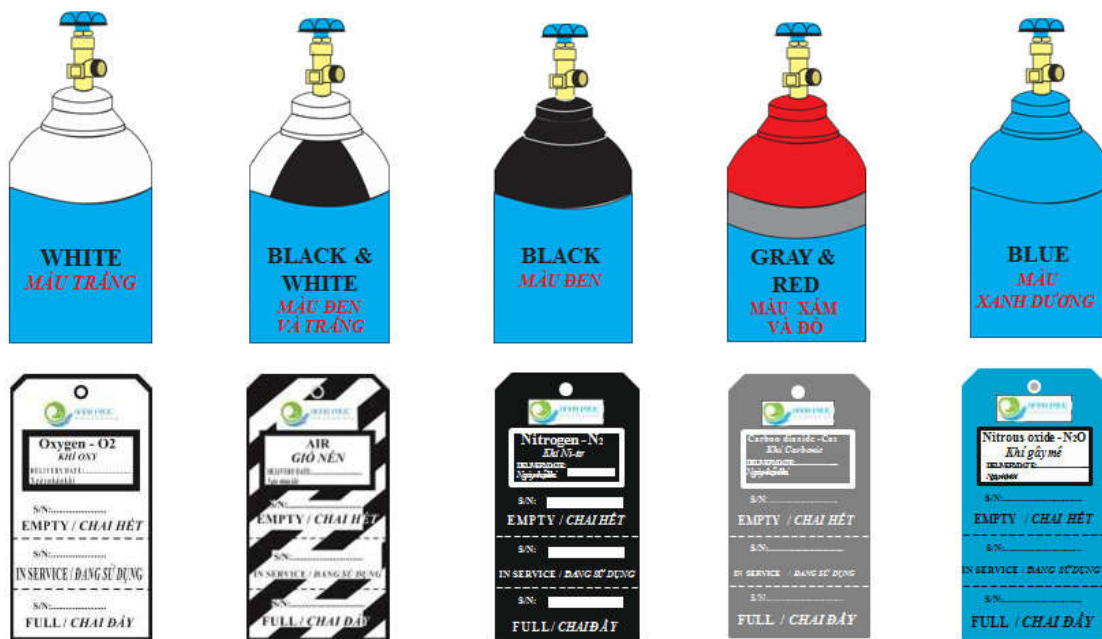
Figure 2: International Medical Gas Cylinder Colour code, adapted in Hanh Phuc International Hospital
