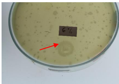
Figure 2: Inhibitory Zone of Biodegradable Antibacterial Activity by Adding Aloe Vera Gel to Staphylococcus aureus Bacteria
