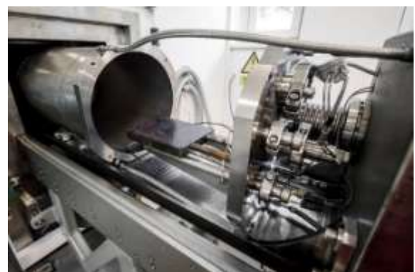
Figure 5: Detailed view of the heating cassette inside the experimental box
