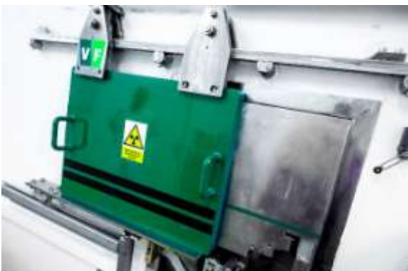
Figure 4: Shielding of the entry to the irradiation chamber
