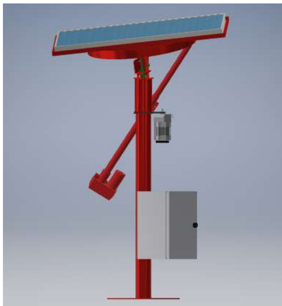
Figure 11: Photovoltaic panel on the solar tracker
