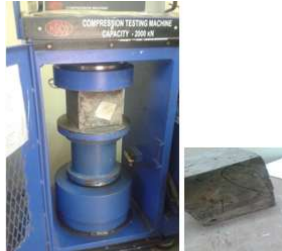
Figure: Testing of Compressive strength test
