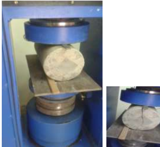
Figure: Testing of Split tensile strength test
