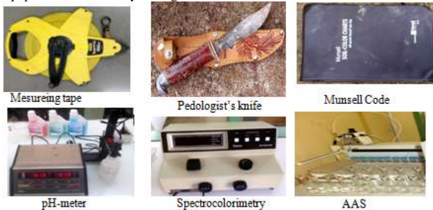
Figure 3: Some elements of soil and laboratory survey equipment
