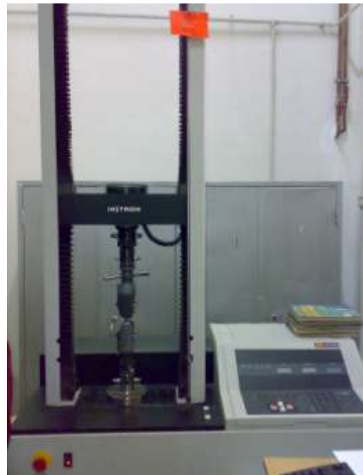
Figure 10 (a): The traction, compression and buckling testing machine Instron 4303.
