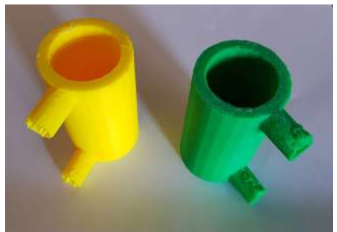
Figure 14: Adhesive will be injected into the plastic fitting in order to perform the assembly through the side controllers
