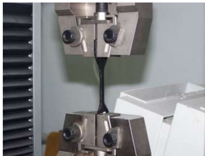
Figure 12: Fastening the pipe in the rams of the testing machine
