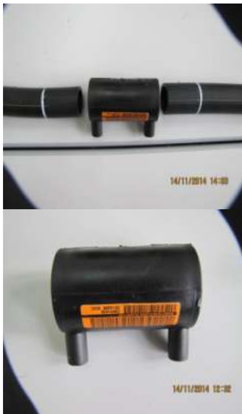
Figure 3: The polyethylene pipe and the fitting before welding
