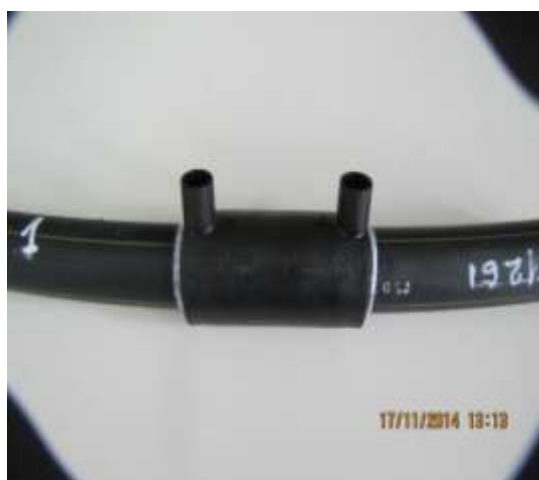
Figure 4: The assembly resulted from electrofusion welding
