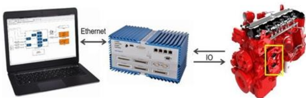
Figure 7: Rapid Control Prototyping Framework
