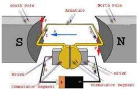
DC motor is an electrical machine that converts electrical energy into mechanical energy(Transducer). It operates at 12V.It consists of Rotor and a Stator. The working principle of DC motor is that "Whenever a current carrying wire or a conductor is placed in the magnetic field, it experiences a mechanical force". A DC motor's speed is controlled over a huge range, using a variable supply voltage or by changing strength of the current in its electric field windings.
