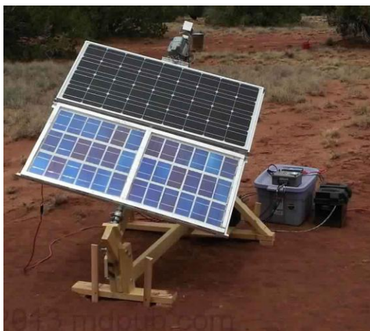
Figure 3: Hardware constructed of VR stepper motor controller for PV System
