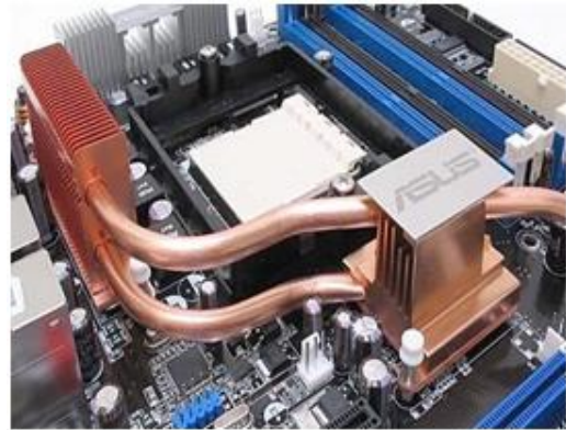
Figure 1.6 Heat Pipe Assembly Used in Mother Board
