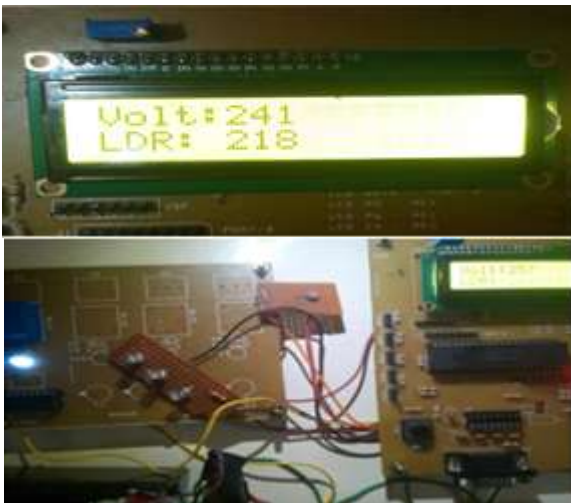
Figure 8: Light intensity is High then relay of LED will not glow
