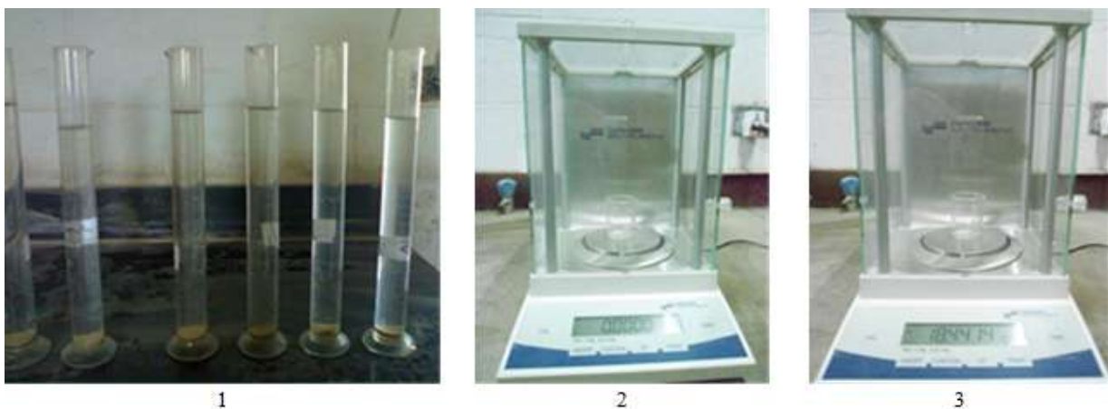
Figure 4: Recommended total dissolved salts test for the soil samples.
