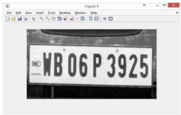
Figure 2 (b): Conversion of original image to grayscale image for using OCR
