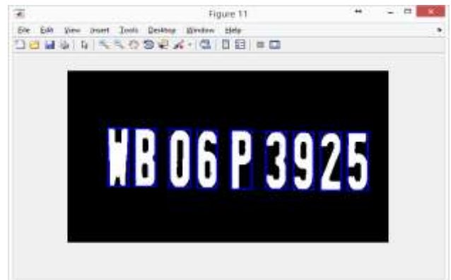
Figure 4 (b): After detection of the characters by bounding box
