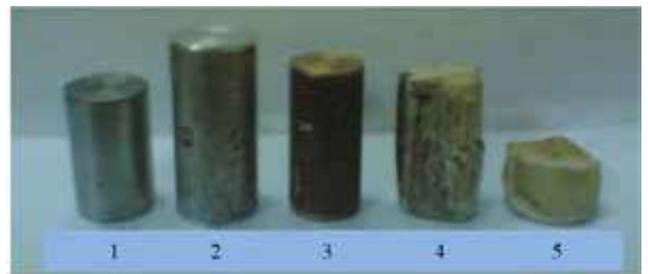
**Figure 5:** Samples for which the speed of sound was measured. 1) Fe, 2) Al, 3) Cu, 4, 5) hard bone
