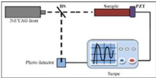
**Figure 1:** Test setup utilized for the photoacoustic system.
