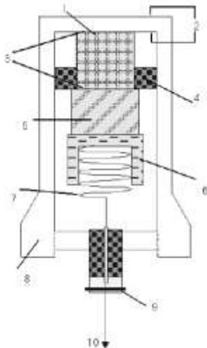
**Figure 3:** Scheme of microphone: 1) piezoelectric(PZT), 2) polished surfaces, 3) silicon grease, 4)hoop of Teflon<sup>TM</sup>, 5) lead 6) copper, 7) spring, 8)stainless steel, 9) BNC connector, 10) to oscilloscope
