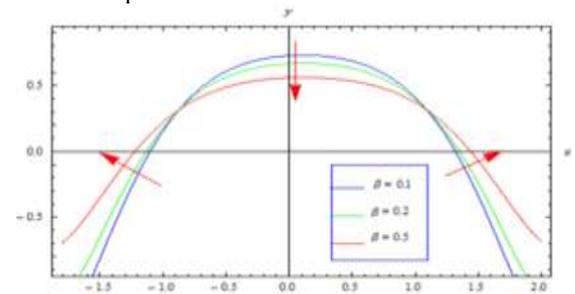
**Figure 4:** Variation of axial velocity  $u$  for different values of  $\beta$  with  $Da = 0.1, H_a = 0.1, a = 0.5, b = 0.4, d = 1,$
