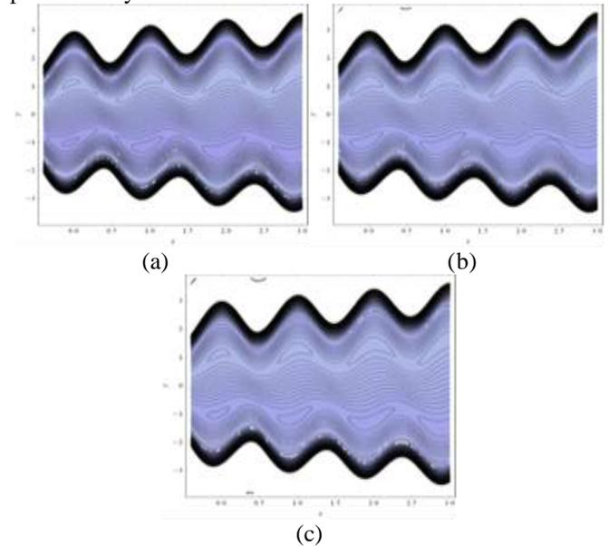
**Figure 20:** Streamlines ( $\psi$ ) pattern for(a) $H_a = 0.1$ , (b) $H_a = 1.6$ , (c) $H_a = 1.8$  with  $Da = 0.1, \gamma = 2, a = 0.5, b = 0.4, d = 1, \beta = 0.1, \phi = \frac{\pi}{4}, F = 1, k = 0.2$
