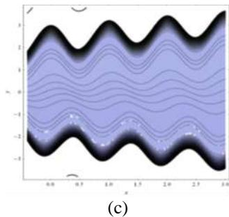
**Figure 22:** Streamlines ( $\psi$ ) pattern for (a)  $\gamma = 2$ , (b)  $\gamma = 2.3$ , (c)  $\gamma = 2.8$  with  $H_a = 0.1$ ,  $Da = 0.1$ ,  $a = 0.5$ ,  $b = 0.4$ ,  $d = 1$ ,  $\beta = 0.1$ ,  $\phi = \frac{\pi}{4}$ ,  $F = 1$ ,  $k = 0.2$
