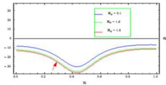
**Figure 8:** Distribution of pressure gradient  $\delta p = \frac{\partial p}{\partial x}$  for different values  $H_a$  with  $Da = 0.1, \gamma = 2, a = 0.5, b = 0.4, d = 1, \beta = 0.1, \phi = \frac{\pi}{4}, F = 1, k = 0.2, y = 1$
