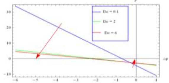
**Figure 15:** Variation of pressure rise  $\Delta P$  with  $F$  for different values of  $Da$  when  $\phi = \frac{\pi}{4}, H_a = 0.1, a = 0.5, b = 0.4, d = 1, \beta = 0.1, \gamma = 2, k = 0.2, y = 1$
