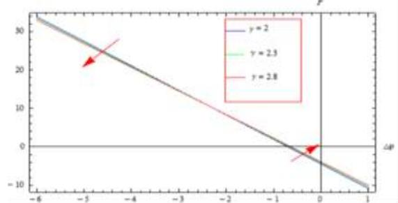
**Figure 16:** Variation of pressure rise  $\Delta P$  with  $F$  for different values of  $\gamma$  when  $Da = 0.1, H_a = 0.1, \beta = 0.1, a = 0.5, b = 0.4, d = 1, \phi = \frac{\pi}{4}, k = 0.2, y = 1$
