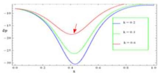
**Figure 13:** Distribution of pressure gradient  $\delta p = \frac{\partial p}{\partial x}$  for different values of  $k$  with  $Da = 0.1, H_a = 0.1, a = 0.5, b = 0.4, d = 1, \beta = 0.1, \phi = \frac{\pi}{4}, F = 1, \gamma = 2, y = 1$
