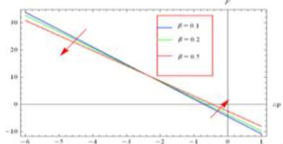
**Figure 17:** Variation of pressure rise  $\Delta P$  with  $F$  for different values of  $\beta$  when  $Da = 0.1, \gamma = 2, H_a = 0.1, a = 0.5, b = 0.4, d = 1, \phi = \frac{\pi}{4}, k = 0.2, y = 1$
