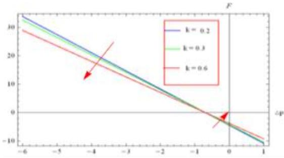
**Figure 18:** Variation of pressure rise  $\Delta P$  with  $F$  for different values of  $k$  when  $Da = 0.1, \gamma = 2, H_a = 0.1, \phi = \frac{\pi}{4}, a = 0.5, b = 0.4, d = 1, \beta = 0.1, y = 1$
