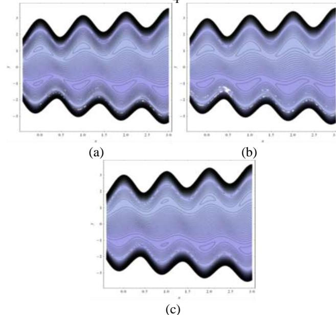
**Figure 23:** Streamlines ( $\psi$ ) pattern for (a)  $\beta = 0.1$ , (b)  $\beta = 0.2$ , (c)  $\beta = 0.5$  with  $H_a = 0.1$ ,  $\gamma = 2$ ,  $a = 0.5$ ,  $b = 0.4$ ,  $d = 1$ ,  $Da = 0.1$ ,  $\phi = \frac{\pi}{4}$ ,  $F = 1$ ,  $k = 0.2$
