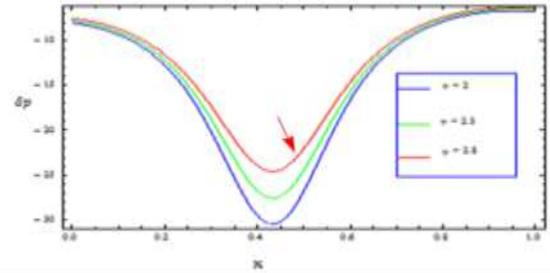
**Figure 11:** Distribution of pressure gradient  $\delta p = \frac{\partial p}{\partial x}$  for different values  $\gamma$  with  $Da = 0.1, H_a = 0.1, a = 0.5, b = 0.4, d = 1, \beta = 0.1, \phi = \frac{\pi}{4}, F = 1, k = 0.2, y = 1$
