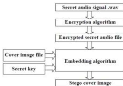
Figure 3.1: Transmitter Flow Diagram
