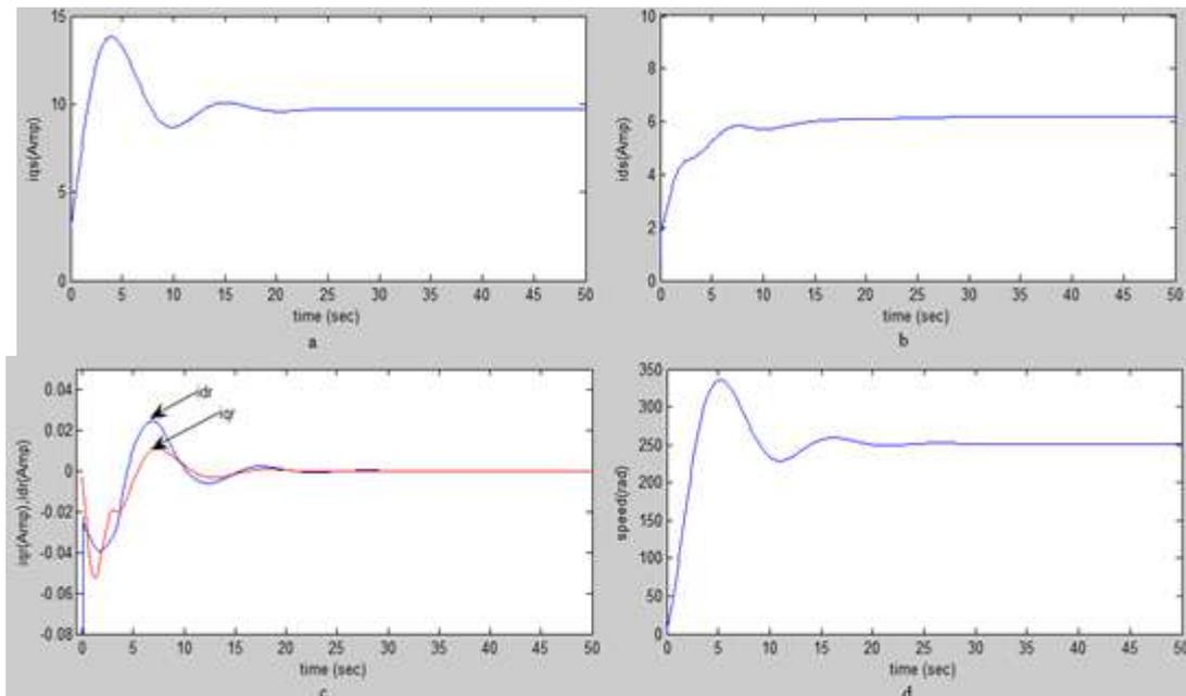
**Figure 6:** Closed loop system Simulation Results of Step change in speed corresponding to a frequency of 40 Hz at constant Torque of the proposed Nonlinear Controller
