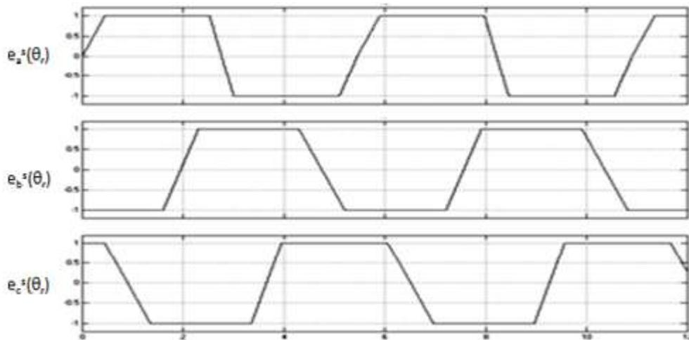
Figure 5: Trapezoidal Induced Emfs of Brushless DC Motor
