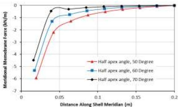
**Figure 14:** Meridional membrane force in the shell along meridian for different half apex angle ( $\alpha$ ).
