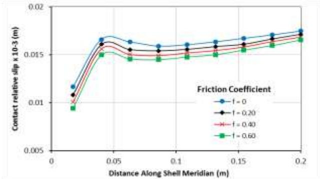
**Figure 8:** Variation of the contact relative slip along meridian
