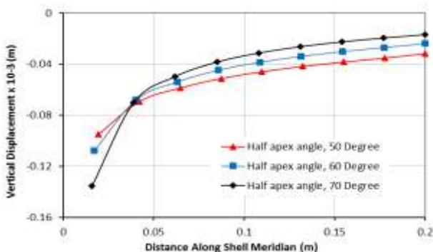
**Figure 13:** Shell vertical displacement along meridian
