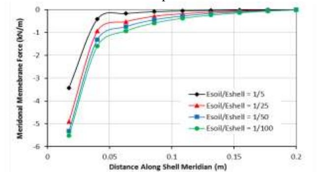
Figure 20: Variation of meridional membrane force in the shell for different Esoil/Eshell ratios.
