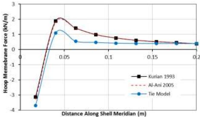
**Figure 7:** Variation of the hoop membrane force in the shell along meridian.
