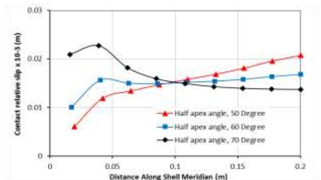
**Figure 16:** Variation of the contact relative slip along meridian for different half apex angle ( $\alpha$ ).
