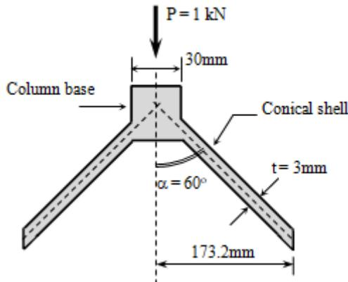
**Figure 3:** Analyzed conical shell footing layout.
