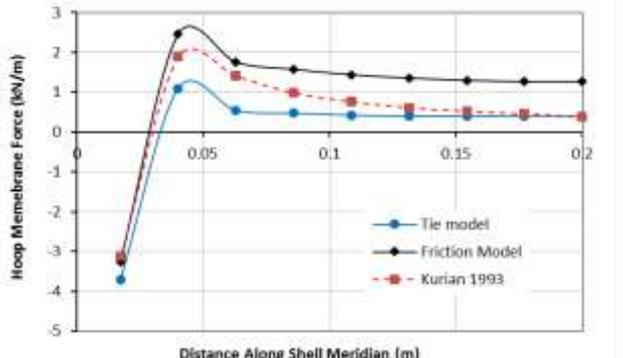
**Figure 12:** Hoop membrane force in the shell along meridian for different analysis models
