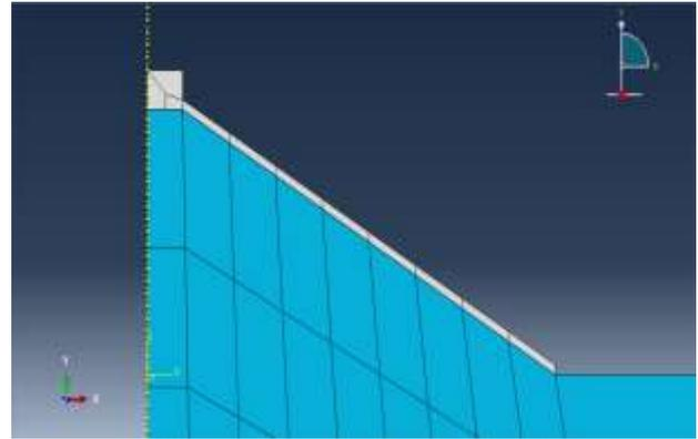
**Figure 4:** Axi-symmetric finite element model for the conical shell footing.
