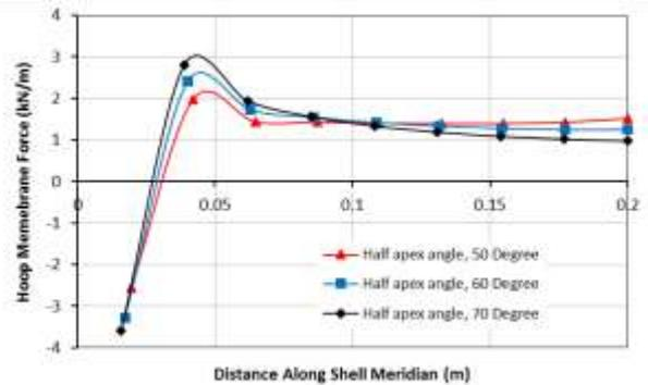
**Figure 15:** Hoop membrane force in the shell along meridian for different half apex angle ( $\alpha$ ).
