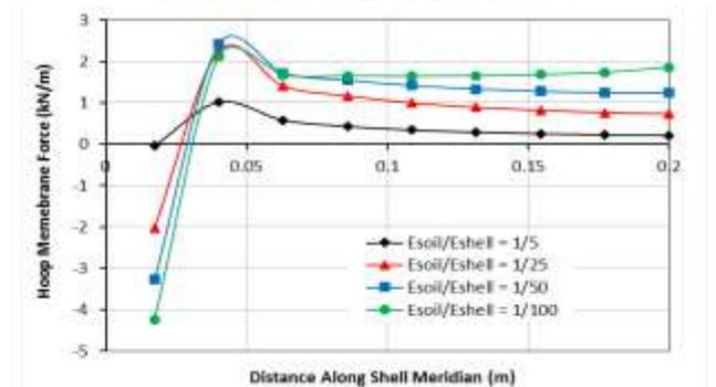
Figure 21: Variation of hoop membrane force in the shell for different Esoil/Eshell ratios.
