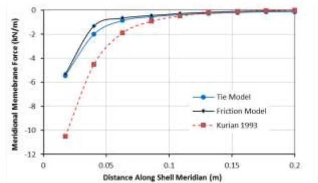
**Figure 11:** Meridional membrane force in the shell along meridian for different analysis models.
