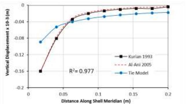
**Figure 5:** Shell vertical Displacement along the meridian.
