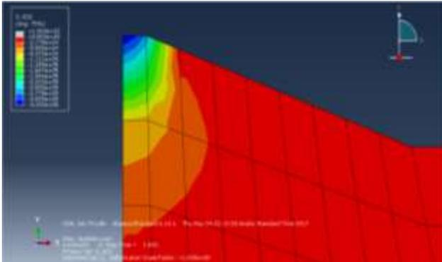
Figure 18: Vertical pressure distribution in the core soil below conical shell for half angle  $\alpha=70^\circ$ .
