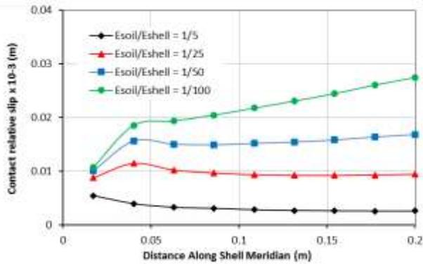
**Figure 22:** Variation of the contact relative slip along meridian for different Esoil/Eshell ratios.
