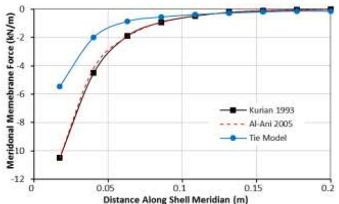
**Figure 6:** Variation of the meridional membrane force in the shell along meridian.
