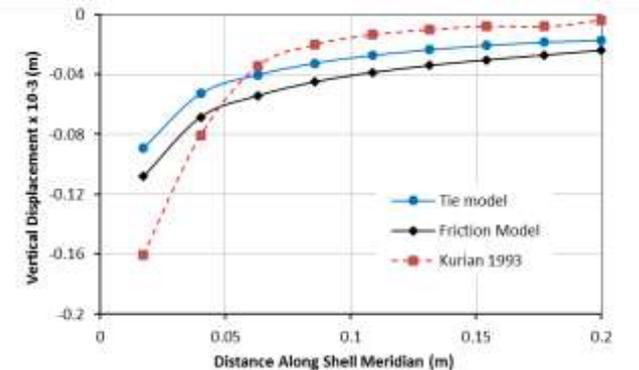
**Figure 10:** Shell vertical displacement along meridian for different analysis models.
