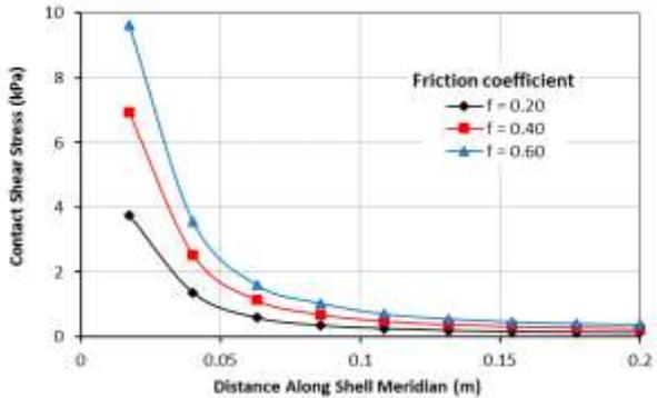
**Figure 9:** Variation of the contact shear stresses along meridian
