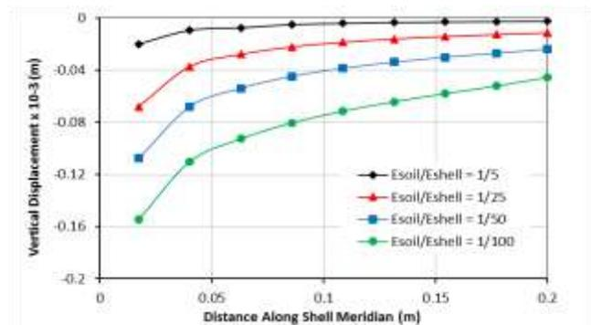
Figure 19: Effect of variation of Esoil/Eshell ratio on shell vertical displacement.
