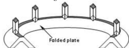
Figure 2: Folded plate footing.
