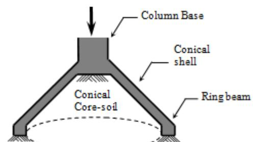
Figure 1: Typical conical shell footing.
