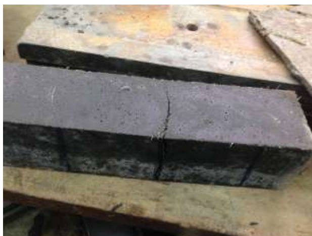
Figure 12: Mode of failure for prism for (RPC)
