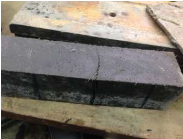
Figure 12: Mode of failure for prism for (RPC)
