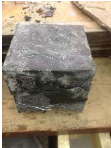
Figure 8: Mode of failure for reactive powder concrete with end hooks steel fibers.
