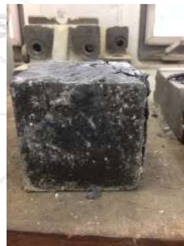
Figure 9: Mode of failure in compression of (RPC) with micro steel fibers
