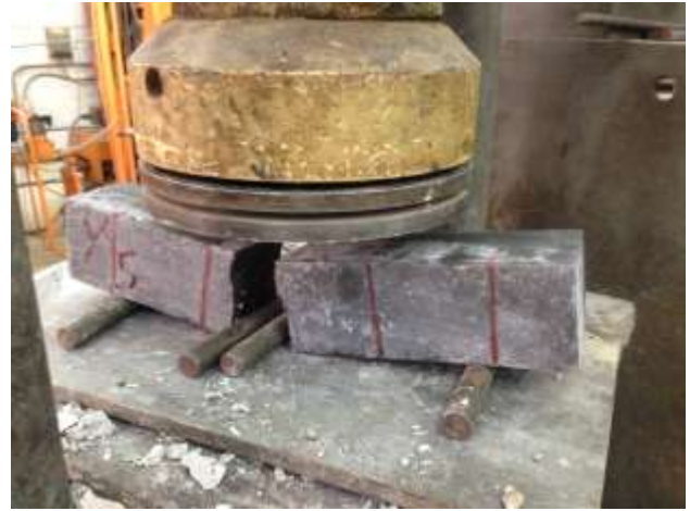
Figure 11: Mode of failure in (RCP) for prism.
