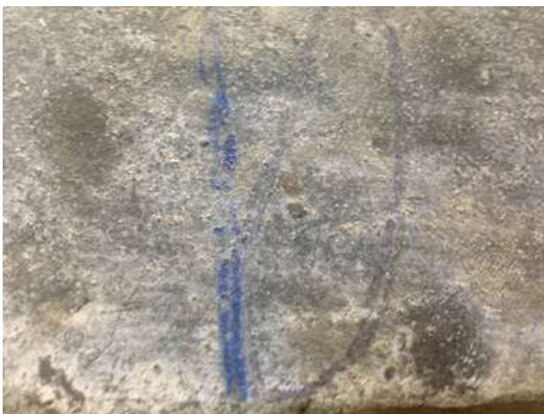
Figure 13: Mode of failure in (RPC) cube with micro steel fiber
