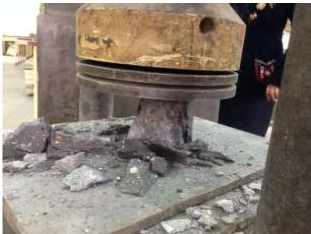
Figure 7: Mode of failure for reactive powder concrete without steel fiber.
