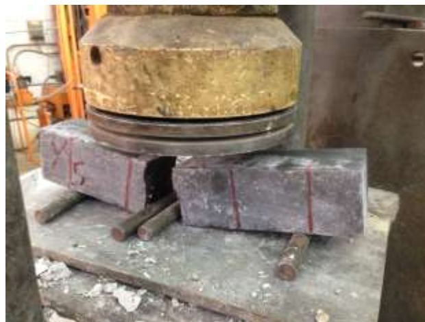
Figure 11: Mode of failure in (RPC) for prism.
