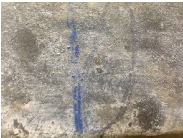
Figure 13: Mode of failure in (RPC) cube with micro steel fiber
