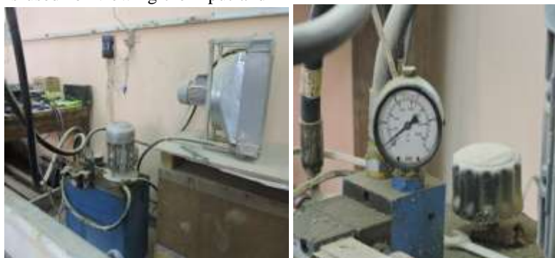
Figure 4: The hydraulic control system
