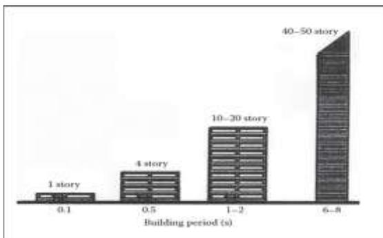
**Figure 5:** Effect of building height on vibration period [1]
