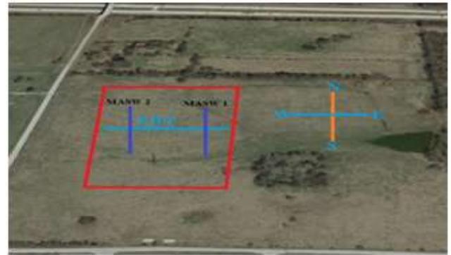
Figure 2: ERT East-West traverse and MASW North-South, courtesy to google earth.
