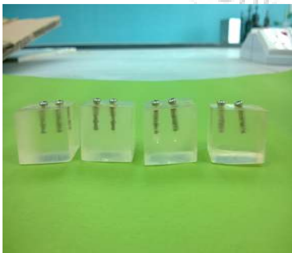
Figure 1: Acrylic master models with implant analogs at different angulations; block a: 0° & 0°, block b: 0° & 5°, block c: 0° & 10°, block d: 0° & 15°.
