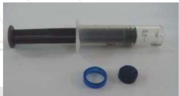
Figure 1: Mould for fabricating wax discs).
