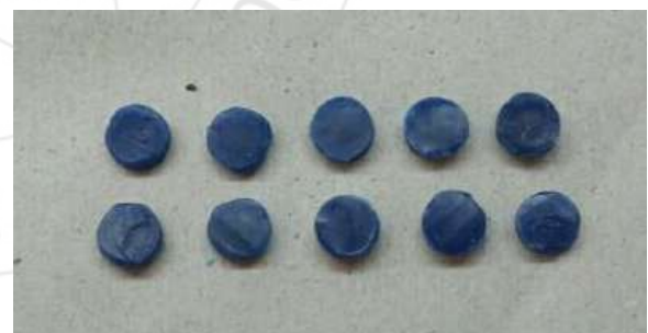
Figure 2: Wax samples fabricated for casting).
