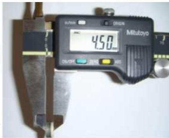
Figure 5: Digital vernier caliper used to measure thickness of the samples
