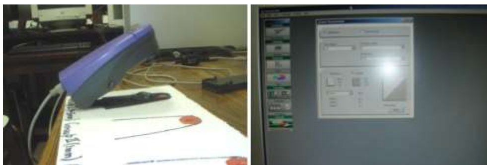
Figure 7: spectrophotometer used for color measurement)
