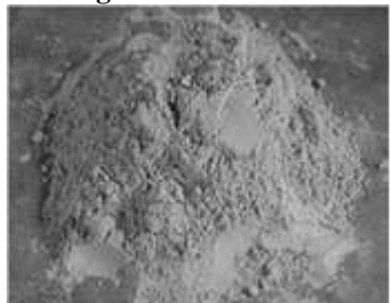
Figure 2: RHA sample after 30 minutes of grinding
