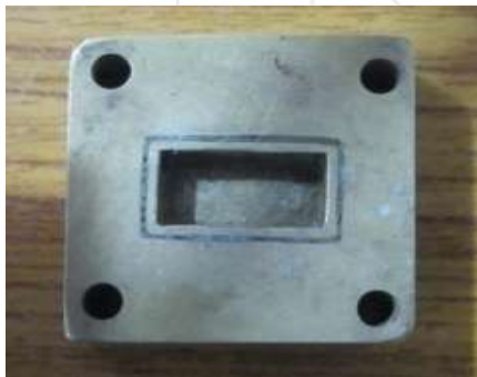
Figure 3: Sample Holder (Ku-Band from 12.4-18.0 GHz)
