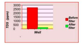
**Total Hardness (T.H):** The removal efficiency was (96.8%) with an average concentration of inlet water (1500 ppm) and product water (48 ppm). Reverse Osmosis membrane is able to reduce water hardness, but the high level of hardness can adversely affect RO membrane and reduce its life as it is quickly fouled by hard water. Therefore, pre-filter must be used such as activated carbon filter to protect the RO membrane [17].
